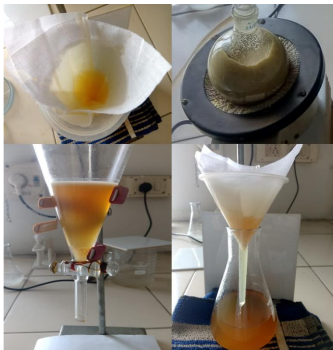
Figure 3. Isolation of essential oil. The resulting hydrodistillation distillate was filtered and transferred into a separating funnel to isolate the lighter upper lipidic layer from the denser lower aqueous phase.
