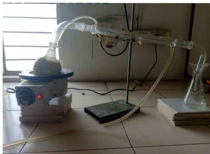
Figure 2. Essential oil extraction setup. The pulverized dried peel samples were subjected to hydrodistillation utilizing a temperature-controlled heating mantle and standard condensation apparatus
